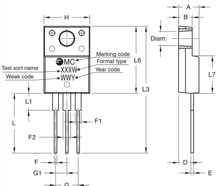
The drawing shows a TO-220F package with a top view and a side view. The top view includes dimensions H, L1, L, F, G1, and G. The side view includes dimensions A, B, L7, D, and E. A marking code is shown on the top view: MC (Fagor logo), XXXW (Format type), WWY (Year code), and Test sort name/Week code. A diameter dimension is also indicated.
