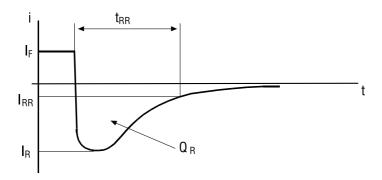
The actual time required for recovery will vary depending on the amount of forward current passed before switching, frequency of switching, waveform (sine, sawtooth, square), impedance of recovery current loop, reverse voltage applied, temperature, and most important, the type of rectifier used in the circuit.
